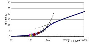
Figure 11 Spalding fit to dual velocity measurements using the Dual Velocity sensor
