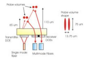
Figure 6 Design of the Dual Microvelocimeter with two probe volumes, one probe volume located at 65  $\mu m$  and a second probe volume located at 110  $\mu m$  above the surface of the sensor.
