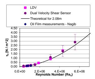
Figure 12 Wall shear stress measurements with the Mini LDV, the Diverging Doppler sensor and oil film interferometry.
