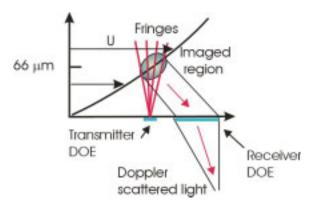
Figure 1 Schematic of the optical shear stress sensor principle of measurement.
