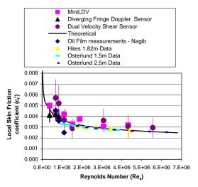
Figure 13 Comparison of local skin friction measurements obtained with the diverging Doppler sensor, the dual Velocity sensor, LDV, oil film, and additional results obtained by Österlund<sup>9</sup> and Hites<sup>10</sup>.
