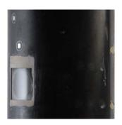
A custom cylindrical enclosure containing a traversing miniLDV and two microS for flow separation studies.
