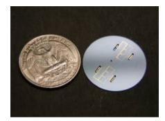
Figure 2 : Array of pressure sensors fabricated by Rheosense Inc.
