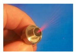
Figure1 : Image of the MicroS3 shear-stress sensor.
