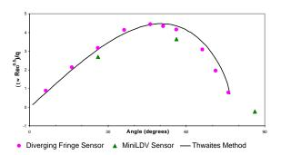
Figure 5 - Measured Wall Shear around a Circular Cylinder
