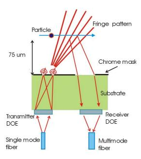
Figure 2 - Diverging Fringe Velocity (dfv) Sensor
