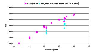
Figure 8 - Variations of flow velocity with Polymer flow rate (at Z = 150 microns)
