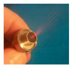
Figure 3 - Photograph of a Diverging Fringe (df) Doppler Velocity Sensor
