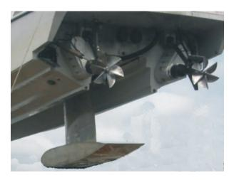
Figure 10 - SDV 45 ft boat with the attached hydrofoil
