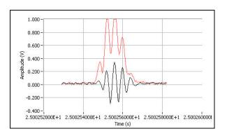
Figure 4 - Typical Doppler signal for diverging fringe velocimeter
