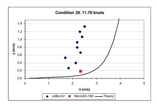
Figure 13 - Measured flow velocity with polymer injection
