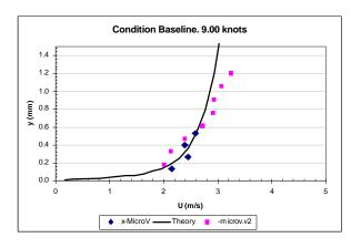
Figure 12 - Velocity data obtained with no polymer injection
